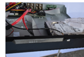
Figure3-1 Installing hard disk
