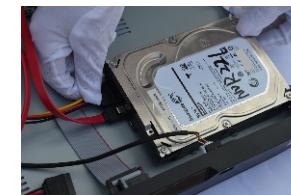
Figure3-2 Insert hard disk data cable and power cable
